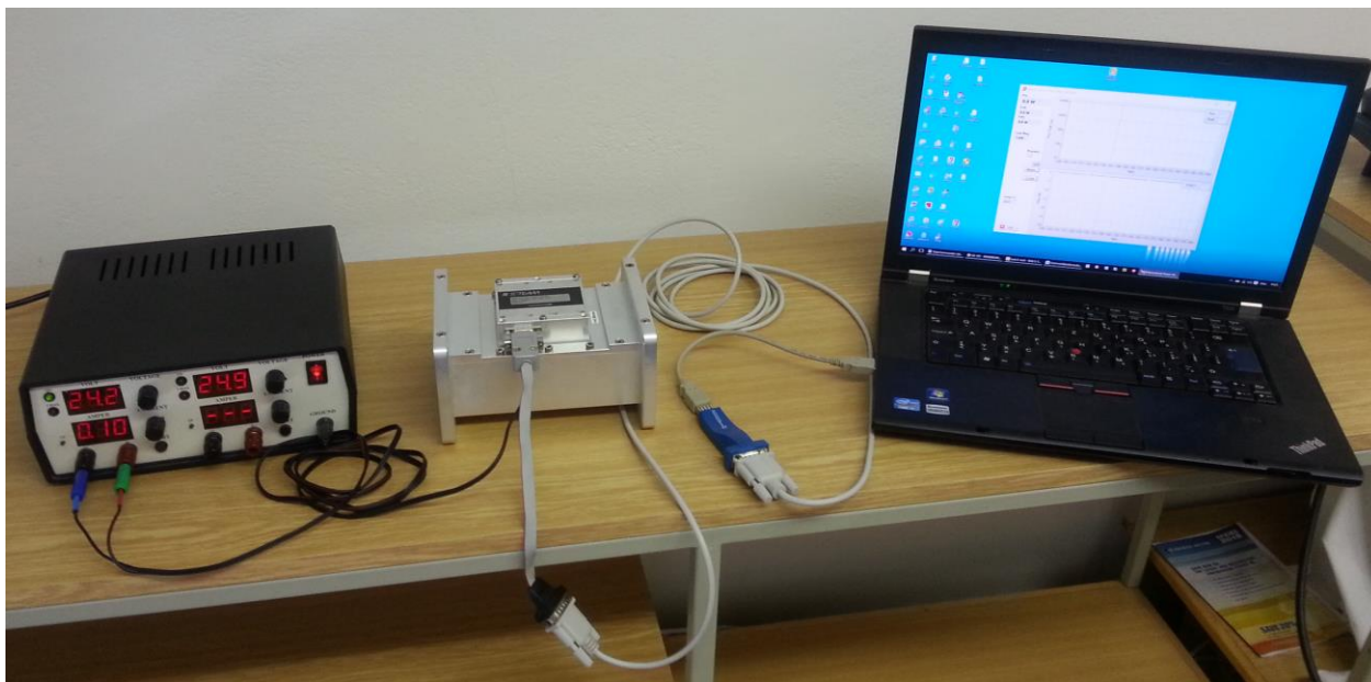
Fig. 15. Illustration of BPM – PC connection.
