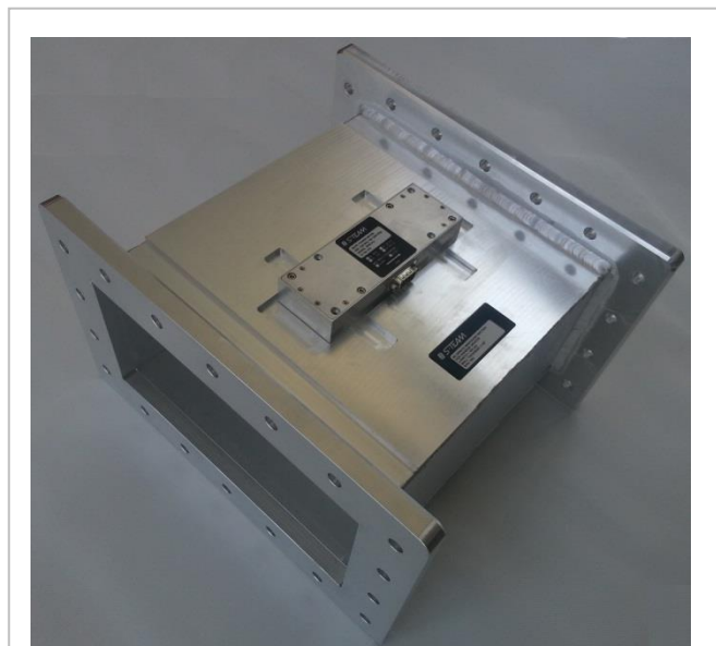
Fig. 2. BPM214 (version without LCD display) installed on the standard-length waveguide.
